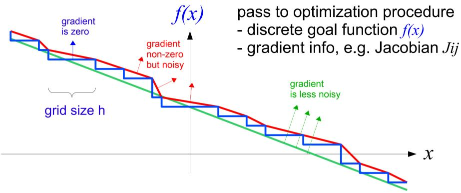
f(x) goal function implemented using chip simulation: zero gradient
