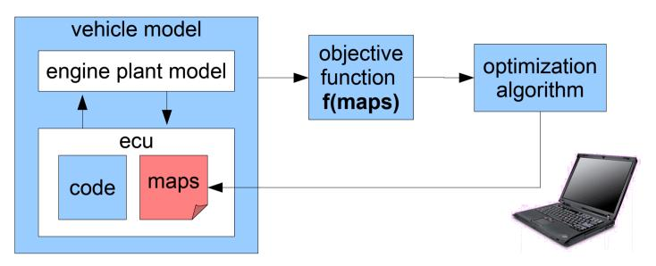
ECU source (C, Ascet, or Simulink model) typically not available for OEM
